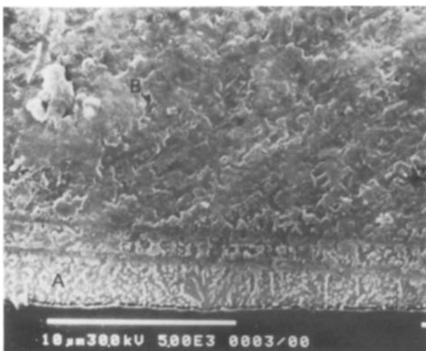
Figure 2 Scanning electron micrograph through the thickness of the as-melt-spun ribbon.
